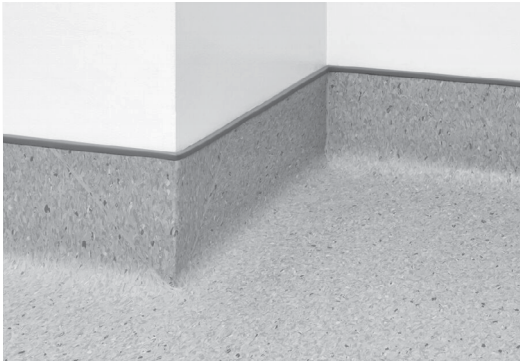
In clinical settings where infection control is a priority, iQ's flexible material can be formed to create an integral cove base between the floor and wall with a gentle radius to prevent accumulation of dust and dirt.
